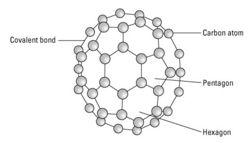
The most common buckyball contains 60 carbon atoms and is sometimes called C60. Other sizes of buckyballs range from those containing 20 carbon atoms to those containing more than 100 carbon atoms.
